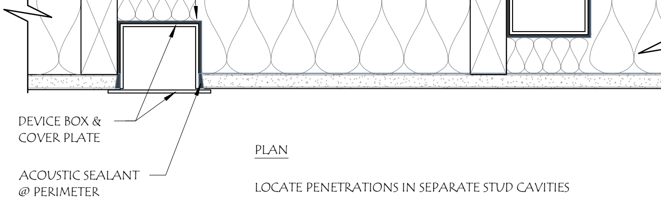
11 ACOUSTIC PARTITION PENETRATIONS SCALE: 1 1/2" = 1'-0"
